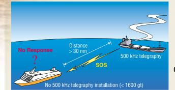
It was only possible for a vessel in distress to ask other vessels in the vicinity for assistance, due to the limited range of communication means.
