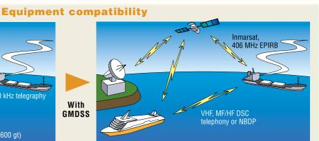
Since all GMDSS vessels carry standardized equipment for the Sea Area, and they are operating in the same frequencies, the compatibility between the SAR coordinator at a coastal station and a vessel is assured.
