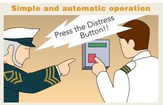
GMDSS equipment, on the other hand, provides straightforward operation in time of emergency simply by pressing the distress button on the VHF, MF/HF DSC or Inmarsat MES. If this cannot be done, a float-free EPIRB can transmit a distress alert.
