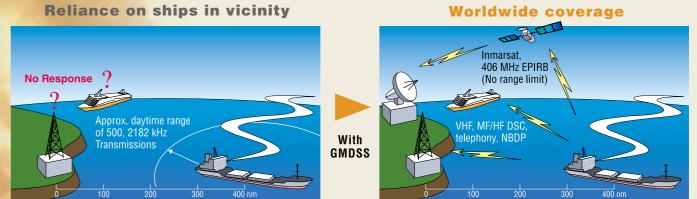
Because of the inherently limited range of transmission on the distress and calling frequencies of 500 and 2182 kHz, which were commonly used for that purpose, there was a possibility that a call for assistance would not be heard if other vessels and coastal stations were outside the range.
